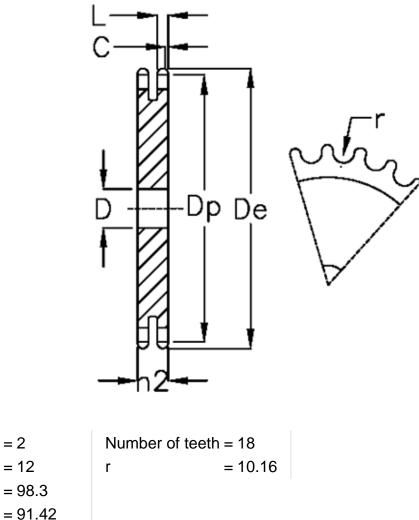
C = 2 D = 12 De = 98.3 Dp = 91.42 For chain size =  $5/8 \times 3/8$ For chain type = 10 B-2 h2 = 25.5 L = 9
